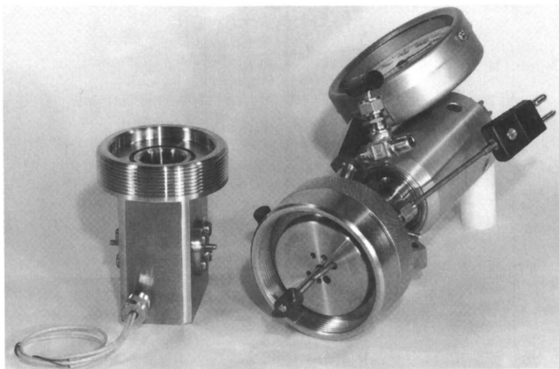
Figure 1. Cylindrical internal-reflectance (CIR) reactor, showing the 50-mL internal-volume autoclave equipped with a high-speed stirrer, thermocouple, high-pressure gauge, base-mounted cartridge heater, and high-pressure seal for the cylindrical internal-reflectance crystal.
