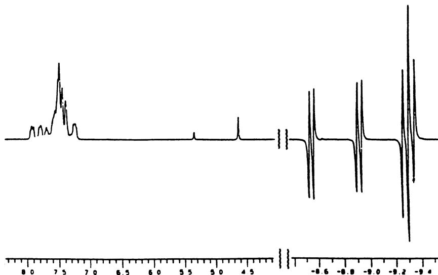
Figure 11. ^1\text{H} NMR spectrum at 400 MHz of \text{IrH}_2\text{Br}(\text{CO})(\text{dppb}) formed in the reaction of \text{IrBr}(\text{CO})(\text{dppb}) with \sim 3 atm of para -enriched \text{H}_2 in \text{CD}_2\text{Cl}_2 at 48^\circ\text{C} , 40 s after thawing from -196^\circ\text{C} . (Reproduced from reference 46. Copyright 1989 American Chemical Society.)
